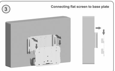
Attach the connecting plate to the base plate.
