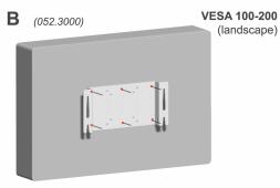
Mount the connecting plate at the back of the screen using the VESA 200-100 mounting holes (landscape). Use the supplied mounting material.
