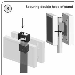
Slide the securing profile over the double head of the stand (when cables come out of the top of the column the cables must be put firstly through the securing profile). The double head of the stand and the securing profile can be locked at the side with an optional anti-theft lock.
