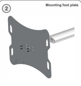
Mount with at least two persons the footplate with 4 bolts (M8x40) to the column. One person is holding the column and the other person is holding and mounting the foot plate. Use a threadlocking fluid to secure the bolts.
